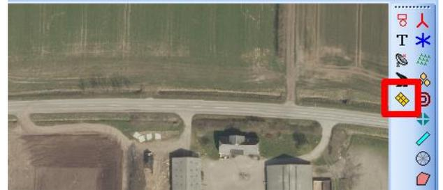
Place the Solar PV object in the area you want to establish solar panels. The exact position is not important, but the map will automatically zoom into the area where the object is placed.
