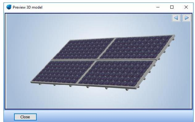
These undividable tables are used to fill out the digitized solar PV area. Increasing the table size, naturally decreases the number of panels fitted to the area.
