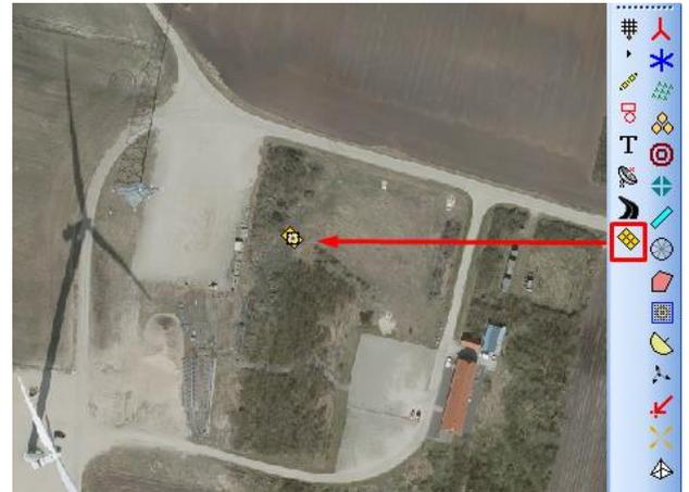
Place the Solar PV object near the area you want to establish solar panels (here we will design a solar plant at the light grey area NW of the WTG). The exact position is not important, but the map will automatically zoom into the area where the object is placed. And it shall be mentioned that the Top of atmosphere radiation is calculated for the location of the object, so it must be “near” the project location.
