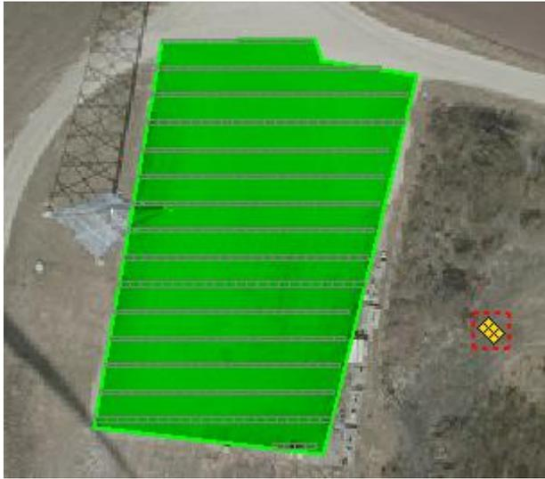
Multiple PV areas and Exclusion areas can be created within the same Solar PV object. Each area can have different properties to the panel layout, panel type and visual design.
