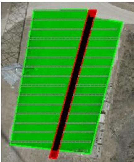
The azimuth follows the general conventions in windPRO, 0 degree is north, 90 degrees is east, 180 south etc. Thus, on the northern hemisphere, 180 degree will make the panels face towards Equator and on the southern hemisphere, 0 degrees will make panels face Equator.
