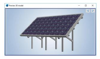
The substructure and panel are two independent components. If we lower the tilt angle of the panel, the substructure does not automatically adjust:
