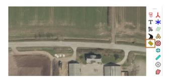
Place the Solar PV object in the area you want to establish solar panels. The exact position is not
