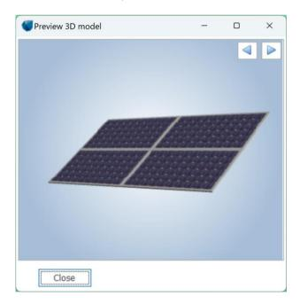
These undividable tables are used to fill out the digitized solar PV area. Increasing the table size naturally decreases the number of tables fitted to the area. Adding more vertical panels usually requires more row spacing.
