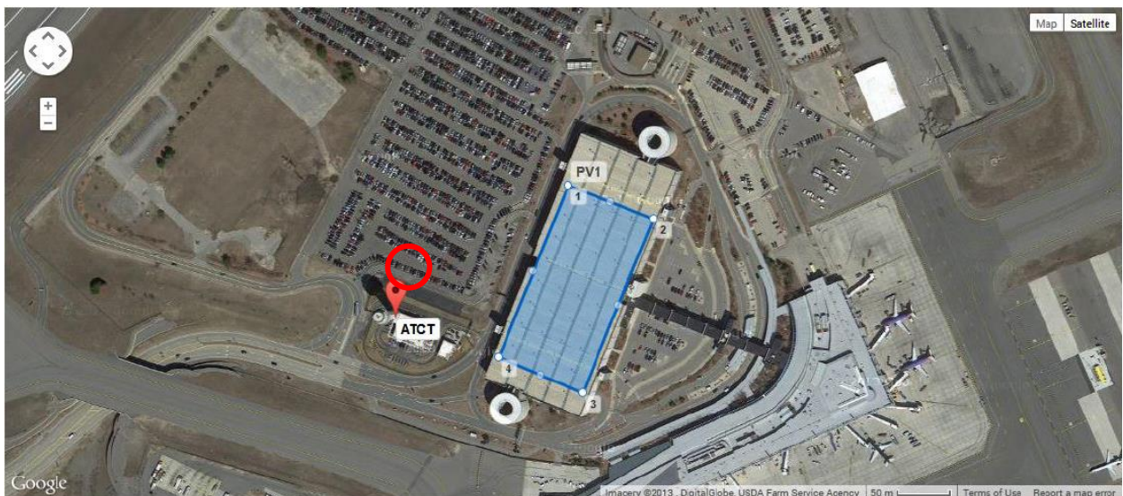
Figure 2 Configuration of the PV plant and glare receptor in SGHAT Tool, the receptor analysed in this comparison marked in red [2]. Map Source: Google Maps.
