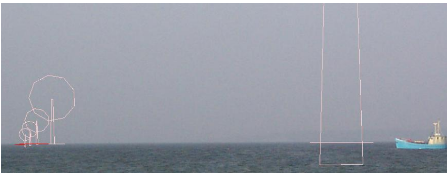
Figure 2 The large rightmost has same colour at the horizon line as the symbol colour: This wind turbine is in front of horizon. The first of the group on the left, is just at the horizon, while the following symbolized with the red colour is behind the horizon. For all turbines the user shall just make sure that the lines follow the horizon, then the rendering takes care of the rest, see next photo with the rendered turbines.
