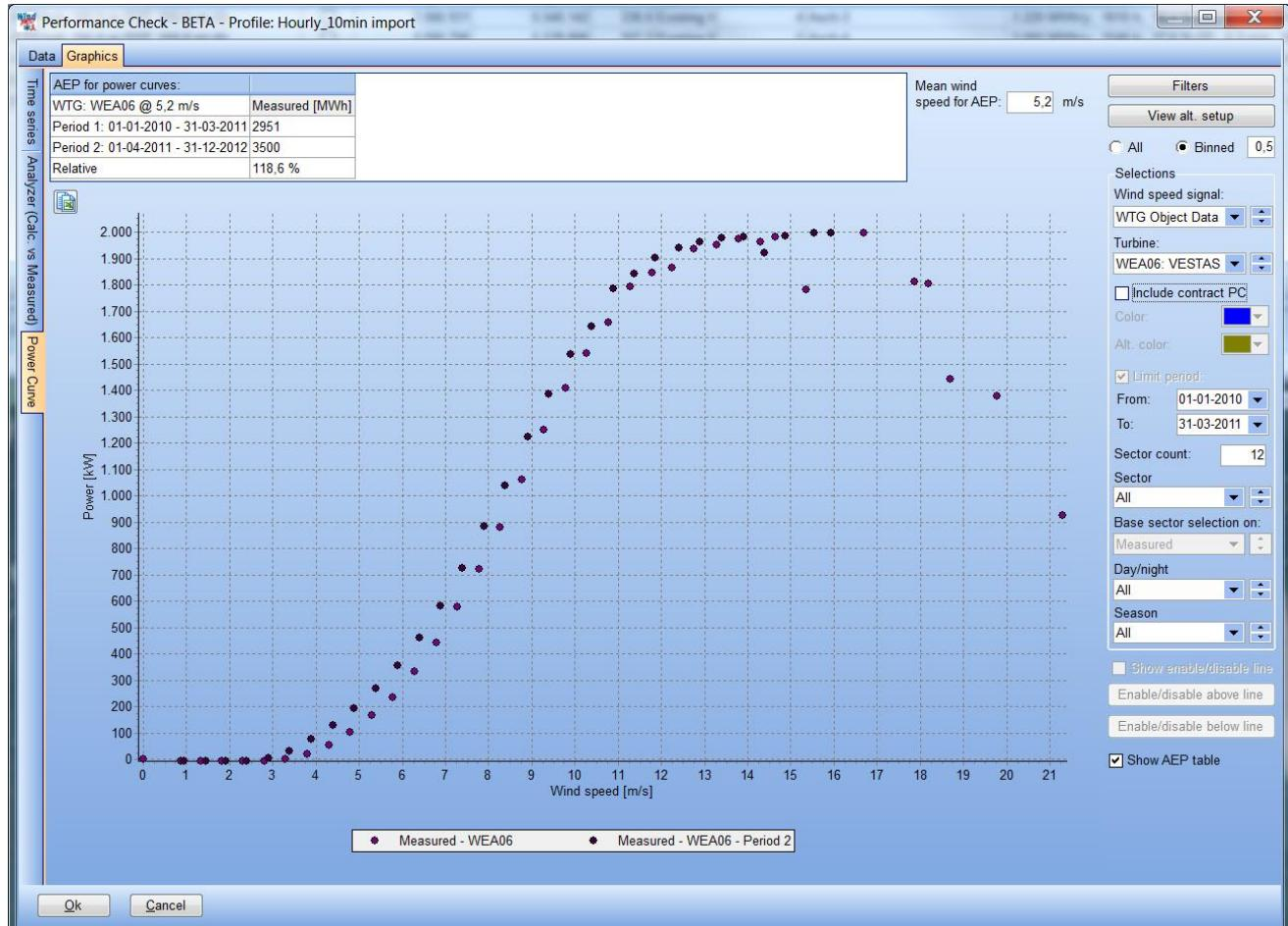
Above is seen an example where two periods are compared. Here it could look as improvement of almost 20%, BUT, based on other analyses, it seem that there has been a modification in the nacelle anemometer calibration between the two periods – and it is not realistic that such large changes are seen.
