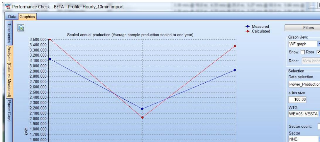
And we do. It's thereby not difficult to conclude that the wake model here does reduce more than it should, and adjustments can be made to wake model settings to get a more precise model setup.
