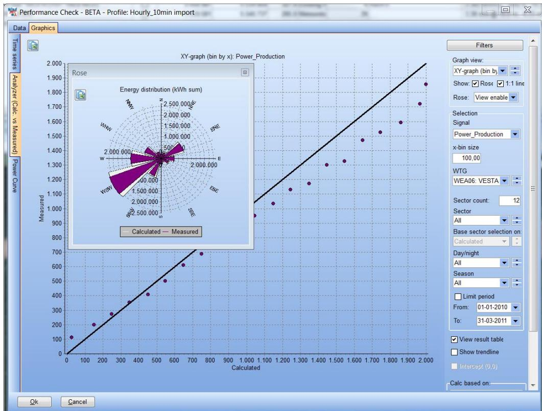
The binned version of the measured vs. calculated show that especially at high production, there seem to be deviations between model calculation and real performance. This might be as well a problem in the used meso scale wind data as a turbine issue or another model based problem.
