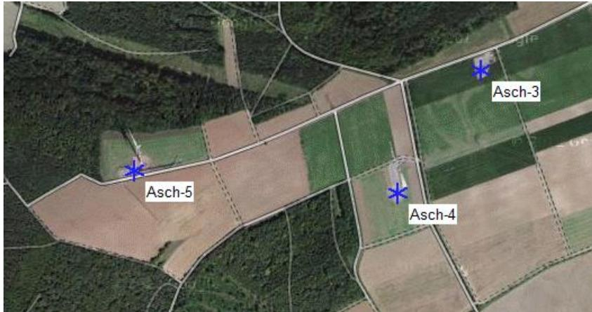
An obvious explanation is that wake losses are calculated too high looking at the wind farm configuration. Especially in SSW, there is much influence from WT-2 (Asch-4) on WT-1(Asch-3). Then we should find similar relative under prediction for Wt-2 in NNE sector:
