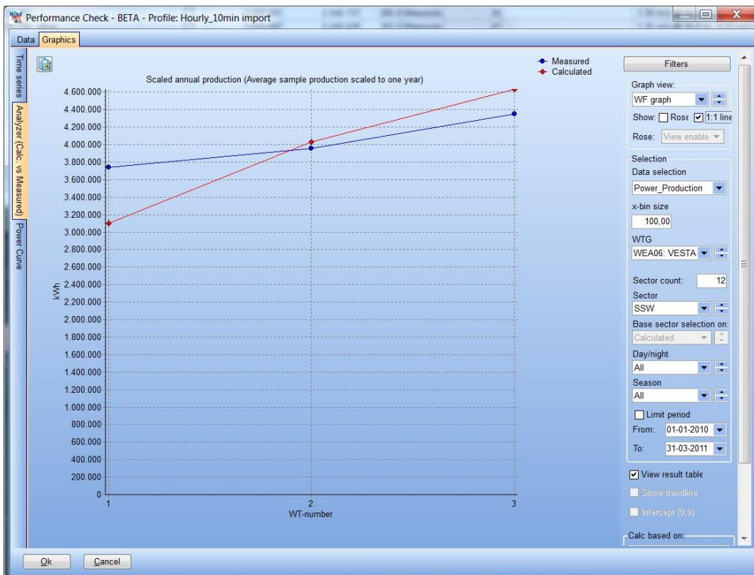
Showing this graph direction by direction complement this further, like in SSW sector, the WT-1 is relative much under predicted.
