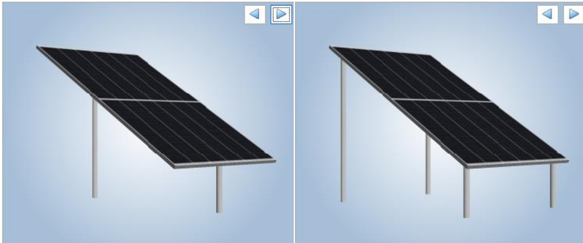
Figure 141 Preview of generic substructures. On the left Count X=1 and Count Y=2, on the right Count X = 2 and Count Y=2.
