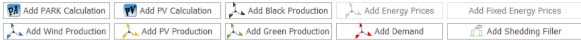
Figure 33 Buttons marked with METEO object symbols require data loaded in METEO objects.
