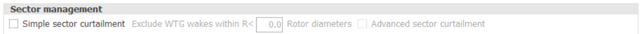
Figure 58. Selection of sector management. Note that Advanced sector curtailment is not selectable, as this option is selected on the SITE COMPLIANCE main tab.
