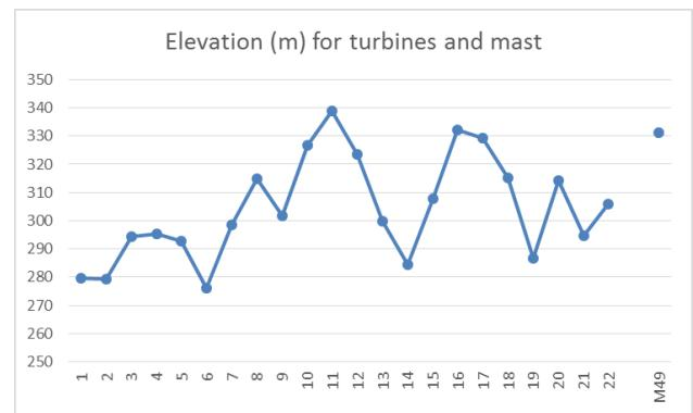
The mast is elevated 25m higher than the average turbine elevation. This can explain why the model might calculate higher AEP than measured, apart from the loss “components” mentioned earlier.
