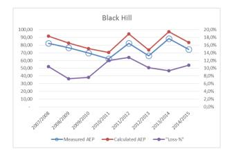
A graphic presentation makes the picture clearer. It is obvious that the mesoscale based calculation catch the annual variations well, but there seems to be an over prediction. Notice, that the calculated production does not include any losses beside wake, while the measured production has losses built into the data.
