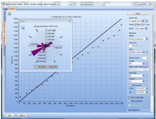
The binned version of the measured vs. calculated show that especially at high production, there seem to be deviations between model calculation and real performance. This might be as well a problem in the used meso scale wind data as a turbine issue or another model based problem.
