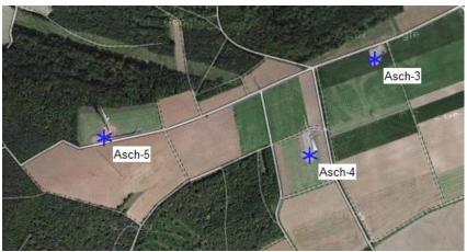
An obvious explanation is that wake losses are calculated too high looking at the wind farm configuration. Especially in SSW, there is much influence from WT-2 (Asch-4) on WT-1(Asch-3). Then we should find similar relative under prediction for Wt-2 in NNE sector:
