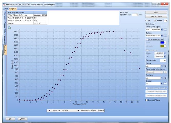
Above is seen an example where two periods are compared. Here it could look as improvement of almost 20%, BUT, based on other analyses, it seem that there has been a modification in the nacelle anemometer calibration between the two periods – and it is not realistic that such large changes are seen.
