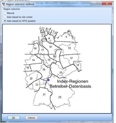
It is seen where the project is located at the index region map, and it is possible to test the neighboring regions by setting the selection to manual and choose the index region. NOTE: The German IWET index is NOT included in the software, the user must paste the data from Excel sheet with the index to the database, but the map is available at EMD online server.
