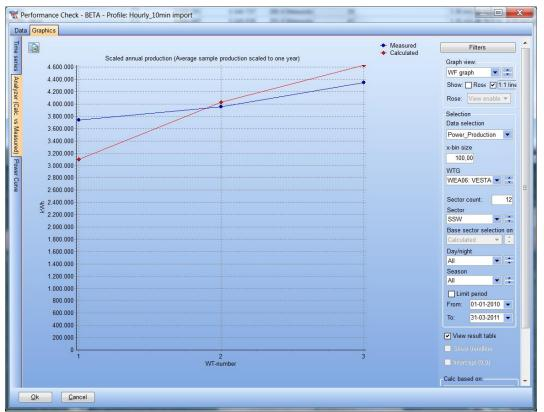
Showing this graph direction by direction complement this further, like in SSW sector, the WT-1 is relative much under predicted.
