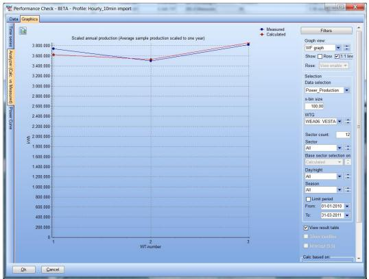
The WindFarm graph show results for all turbines in the same graph. Turbine 1 is slightly under predicted, while the two other match very well. This is an important feed back to the model setup.
