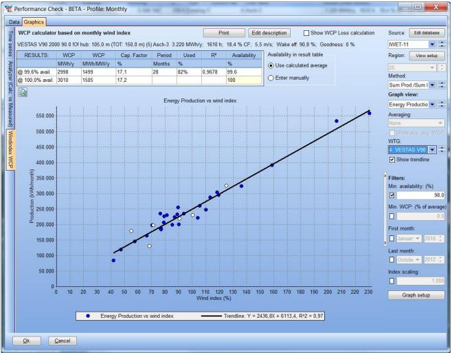
Here is filtered so months with less than 98% availability are excluded in the calculation. This reduces result from 3069 to 3010 MWh (2%) as 100% availability result. Last one is probably more correct, while the low availability in this case seem to be in periods with less wind – in other cases it might be reverse.
