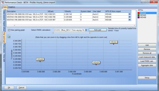
When paired, the button "Load measured data" will transfer the data from the import files to the WTG objects. If having a time varying park calculation **based on same time resolution**, this can be selected and model calculations can be compared to measurements on time stamp level.
