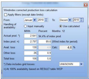
Here the "simple calculated" (from time-avail.loss) availability loss is 4.6%, while the Total loss sum up to 5.6%. This can be explained by stand still periods mainly are in high wind periods in 2010. But it also just could tell that the turbine performance were poorer in 2010 than the next two years for some other reasons – or that the wind energy index not is accurate enough to make the calculation correct.
