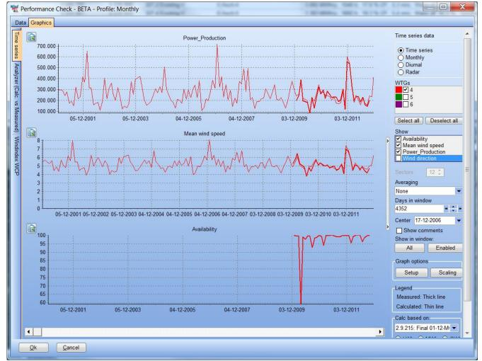
An illustration of monthly data, where a time varying PARK calculation is performed from 2001-12, but where measured production only is available 2009-12. Note also the measured monthly availability is part of the data set. Looking at the time series data it is important to notice that these always will be unfiltered.
