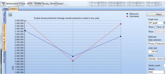
And we do. It' thereby not difficult to conclude that the wake model here does reduce more than it should, and adjustments can be made to wake model settings to get a more precise model setup.
