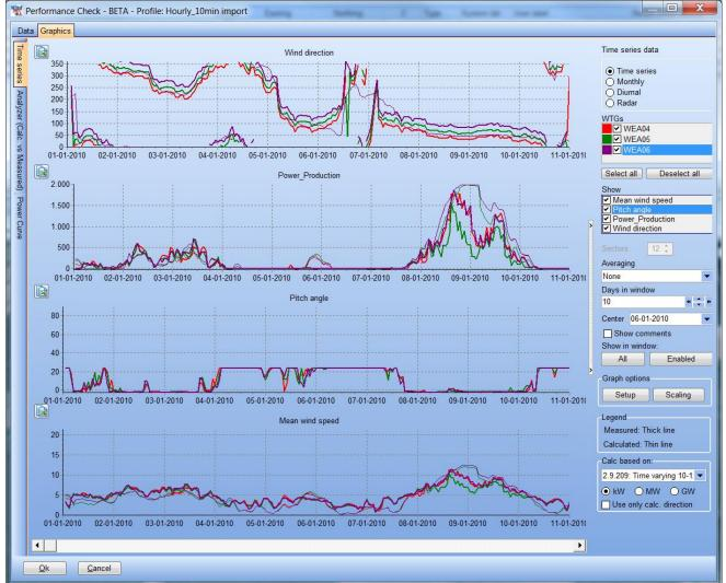
Example on time variation. When both measured and calculated data are shown, the thick line is used for measured, thin for calculated. Example show measured directions are very different. This will often be seen due to the often some primitive system logging the direction of the nacelle. Therefore a checkbox [] use only calculated direction is included.
