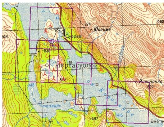
Figure 6 - Five WAsP-CFD tiles defined on a site
