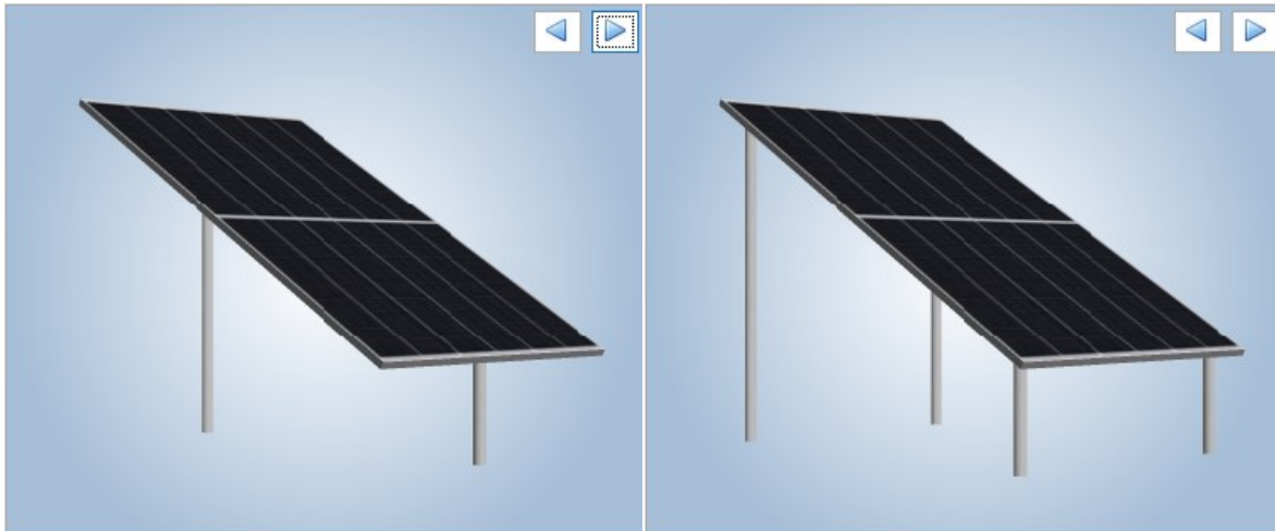
Figure 152 Preview of generic substructures. On the left Count X=1 and Count Y=2, on the right Count X = 2 and Count Y=2.
