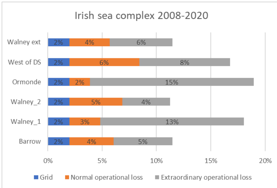
Figure 246 Assumed all time losses in addition to wake losses for the 6 wind farms.
