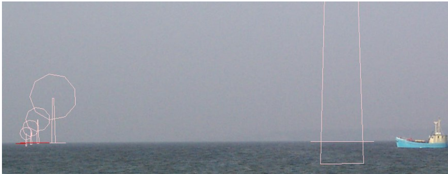
Figure 2 The rightmost turbine has same colour for its horizon line as the symbol colour: This wind turbine is in front of horizon. The first of the group on the left is just at the horizon, while the furthest turbines symbolized with the red colour are below the horizon. For all turbines the user needs to just make sure that the lines follow the horizon, then the rendering takes care of the rest, see next photo with the rendered turbines.
