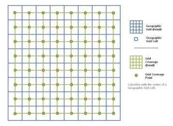
Figure 4: Copernicus DEM grid definition (GTRasterTypeGeoKey = *RasterPixelIsPoint*; figure adapted from [RD-02])
