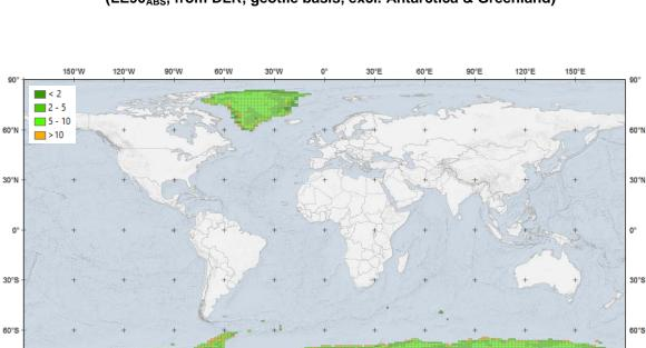
Figure 15: Spatial distribution of absolute, vertical accuracy statistics (LE90<sub>ABS</sub>, from DLR, geotile basis, excl. Antarctica & Greenland)
