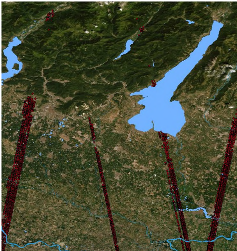
Figure 2: Image of filtered ICESat data (red points) – Lake Garda Northern Italy (Source: Esri World Imagery Basemap)
