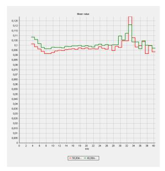
Here, turbulence measurements are available and are used as support for the decision to use the WDC. The average turbulence is observed to be around 0.1, measured close to hub height (47m for this project established).
